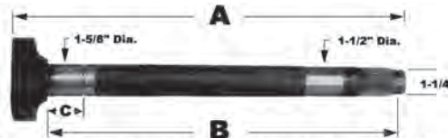
Note: Dimension shown is from shoulder of camhead to far edge of lock ring groove.
