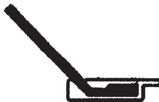
Side Seal Assembly TO-69922
